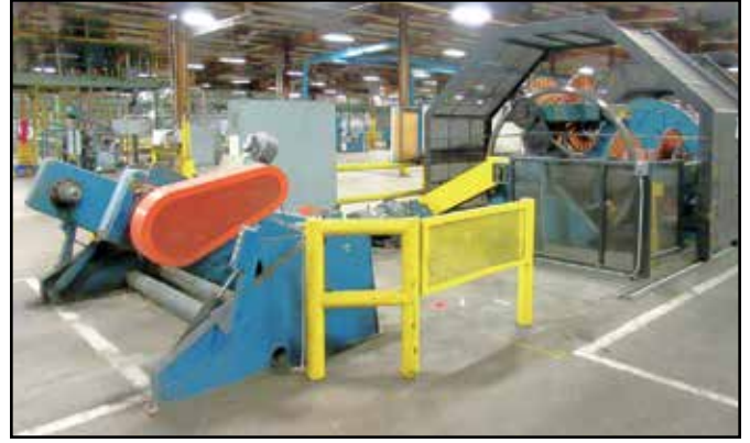
CEECO 48" 3-BAY PLANETARY CABLER LINE
